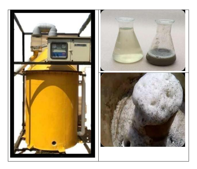
In this stage, further carrying away of **fines** is prevented. The Nano Bubbles being charged help in coalescence of the impurities and this helps in removal and load reduction by removing them in form of foam. There is no membrane, no maintenance it is use of aeration for skimming. The resulting water is free of most of the organic load. Free of fats and milk proteins. The Nano Bubbles being charged also demulsify milk solids from water.
